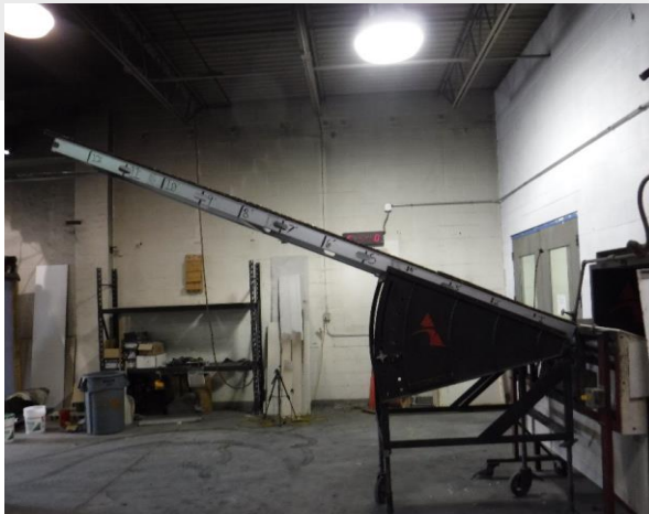
ASTM E108 Class C Fire Test of Roof Coverings
