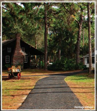
KBI Flexi-Pave also meets and exceeds ADA compliance with a 0.65 coefficient of friction rating.
